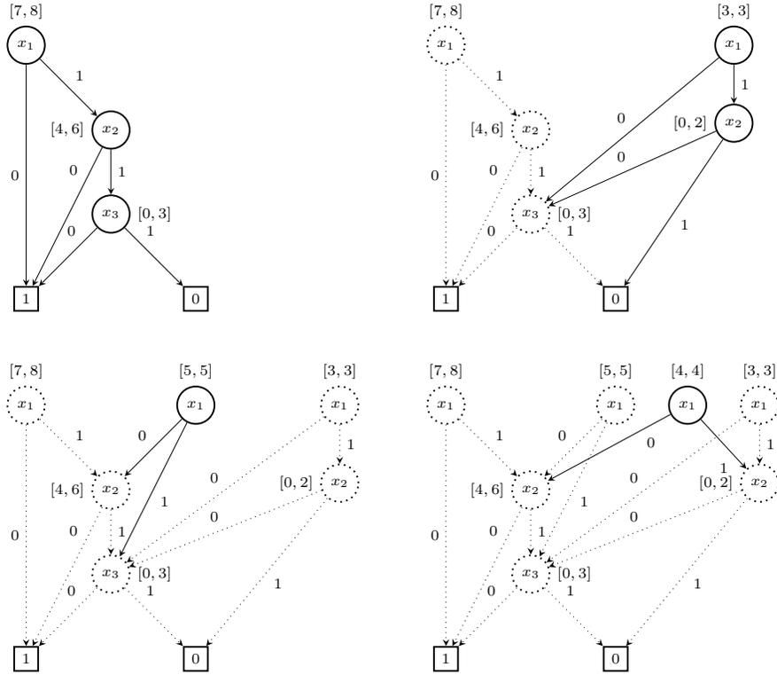
**Fig. 3.** ROBDDs and intervals for  $2x_1 + 3x_2 + 4x_3 \leq 7$  (top left),  $2x_1 + 3x_2 + 4x_3 \leq 3$  (top right),  $2x_1 + 3x_2 + 4x_3 \leq 5$  (bottom left) and  $2x_1 + 3x_2 + 4x_3 \leq 4$  (bottom right), illustrating the reuse of previous ROBDDs.
