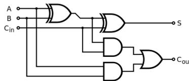
which adds binary numbers and accounts for values carried in as well as out. The code of lines (25-28) employs *n* full adders to obtain a *n*-bit adder. In particular, line (26) defines the output *s* using two *xor* gates, while lines (27-28) model the carries employing two *and* and one *or* gates.
