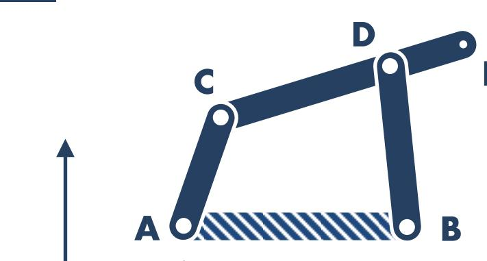
The linkage is fully determined by the coordinates of the fixed pivots A and B and the lengths of the links:
