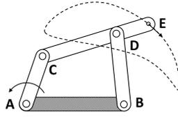
**Fig. 1.** A four-bar linkage and output *coupler curve*
