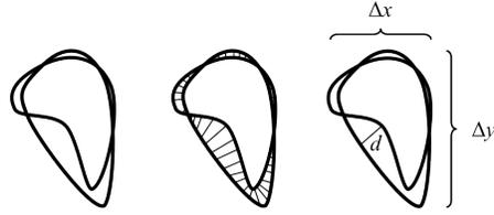
**Fig. 2.** The Hausdorff distance is obtained by finding, for all points on one curve, the closest point on the other, and keeping the distance of the furthest pair. X- and y-dimensions are also shown.
