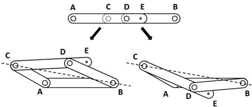
**Fig. 7.** Singular behaviour when  $CD + BD = AC + AB$
