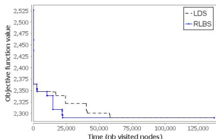
**Fig. 1.** Solution objective function value according to computation time of LDS and RLBS for case #1
