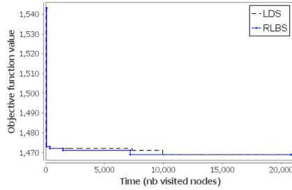
**Fig. 3.** Solution objective function value according to computation time of LDS and RLBS for case #3
