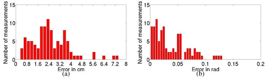
**Fig. 7** (a) Histogram representing the position error made by the bearing-only system for the calibration dataset. The error mean is 2.4947 *cm*. (b) Histogram representing the orientation error made by the bearing-only system for the calibration dataset. The error mean is 0.0370 *rad*.
