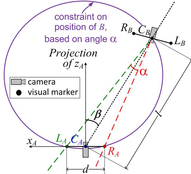
**Fig. 2** Our 3D solution relies partially on a conversion into a 2D localization problem. The reduction in 2D is possible because  $C_A$ ,  $L_A$ ,  $R_A$  and  $C_B$  are all coplanar. Two angles are extracted within this plane: the angle  $\alpha$  between the markers  $L_A$  and  $R_B$  as perceived by  $B$ , and the angle  $\beta$ , between  $C_B$  and the projection of the optical axis of  $A$  onto this plane.
