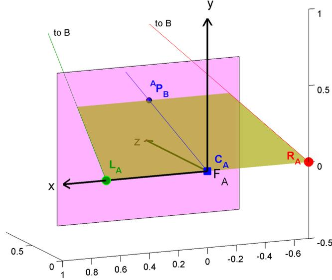
**Fig. 3** The problem, as seen from the camera of *Robot<sub>A</sub>*. The  $z$ -axis, which points away from reader, is the optical axis of the camera. Note that the  $x$ -axis must point left, to respect the right hand rule of Cartesian coordinate systems. The pink surface is the image plane and the point  ${}^A\mathbf{p}_B$  lies within that image plane.
