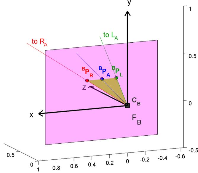
**Fig. 4** The problem, as seen from the other robot *Robot<sub>B</sub>*. The  $z$ -axis, which points away from reader, is the optical axis of camera  $B$ . This camera sees the two markers  $R_A$  and  $L_A$ , as well as the other camera  $A$ . The points  ${}^B\mathbf{p}_R$ ,  ${}^B\mathbf{p}_A$  and  ${}^B\mathbf{p}_L$  all lie within the image plane depicted in pink.
