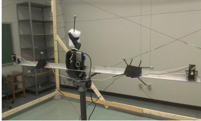
**Fig. 5** Each robot was a long metal rod on which we attached a camera in the center and a LED at each end of the rod. We added multiple OptiTrack markers so the robot could be tracked by the OptiTrack V100:R2 cameras fixed all around the room. The moving robot is on a tripod with a swivel head, and a clamp is firmly holding the metal rod in place.
