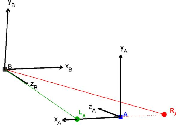
**Fig. 1** The relative localization problem in 3D, for the two robots  $A$  and  $B$  operating in 6 DoF. In this depiction, we only show the markers on robot  $A$ . The red and green lines represent the ray between these markers and the center of projection of  $Camera_B$ , located at the origin of  $F_B$ .
