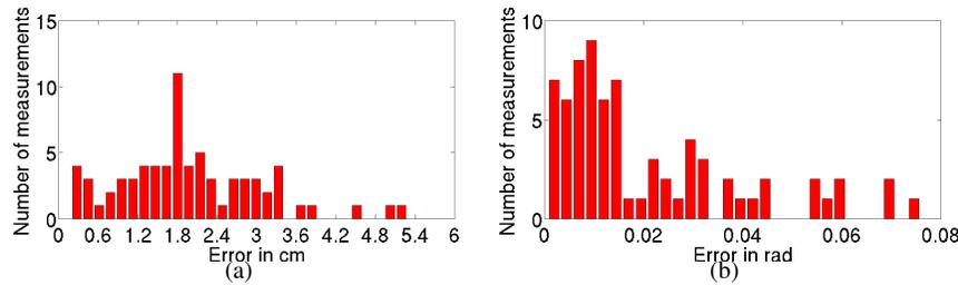
**Fig. 8** (a) Histogram representing the position error made by the bearing-only system for the test dataset. The error mean is 1.9885 *cm*. (b) Histogram representing the orientation error made by the bearing-only system for the test dataset. The error mean is 0.0205 *rad*.
