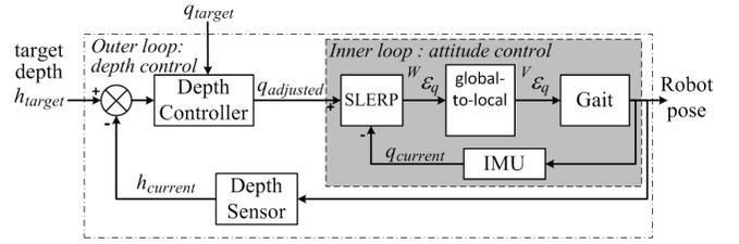
Fig. 4. An overview schematic of our vehicle controller.
