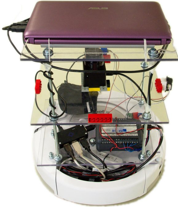
Figure 3. The robot produced in ten copies for the course usage, featuring an 8-channel ADC, a laser rangefinder, two infrared sensors, and a motorized Roomba base. The upper plate was left clear such that students could strap in their own laptop.
