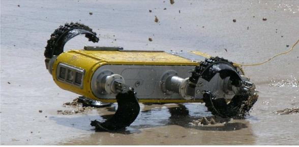
**Fig. 17** The hexapod robot, shown equipped with semi-circle legs for land locomotion. The vehicle moves forward by constantly rotating legs in two groups of three, forming stable tripod configurations.
