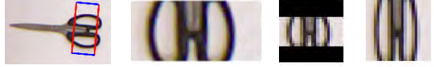
Figure 2. Left: a pair of scissors with a candidate grasp rectangle image. Center-Left: image taken from the rectangle rotated to match the global image orientation. Center-Right: rescaled image with preserved aspect ratio. The black regions indicate masked-out padding. Right: rescaled image without preserved aspect ratio. Preserving aspect ratio reduces distortion.
