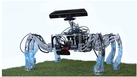
Fig. 1. The Messor robot, used to collect the data sets in the experiments.
