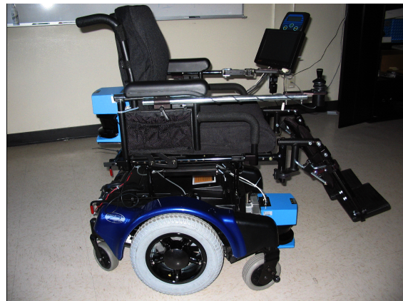
Figure 2: The SmartWheeler robot platform (Pineau et al., 2011).
